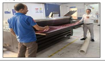
Following washing, the plate is exposed to the Vinord EVO DLF 3000, equipped with a Hot Air Blower to evaporate the chemicals used during washout. During the thermal development plates are exposed with warm air of approx. 60 degrees Celsius.
