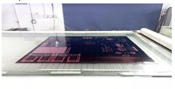
After Thermal Development the plates are exposed to UV-A and UV-C light again to complete photo curing in a combi processor and to eliminate the tackiness of the plate surface.
