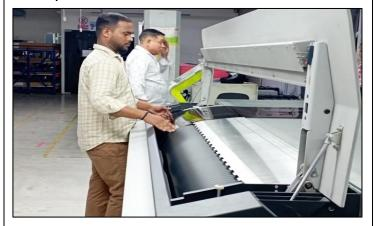
Following image engraving, the plate undergoes exposure in the DuPont Digiflow 3000 ETL machine, where UV A light hardens the engraved or imaged areas of all the flexo plates and metal back plates. This process selectively hardens the plate sections corresponding to the design while keeping other areas soft.
