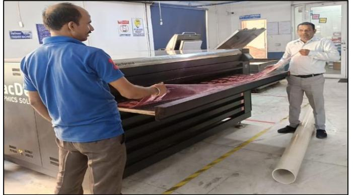
Following washing, the plate is exposed to the Vinord EVO DLF 3000, equipped with a Hot Air Blower to evaporate the chemicals used during washout. During the thermal development plates are exposed with warm air of approx. 60 degrees Celsius.
